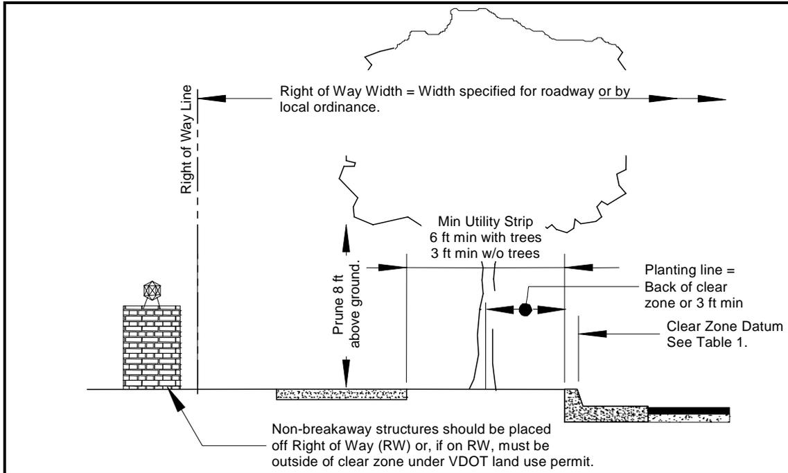
**FIGURE 10 - SETBACK DETAILS WITH CURB AND GUTTER**
