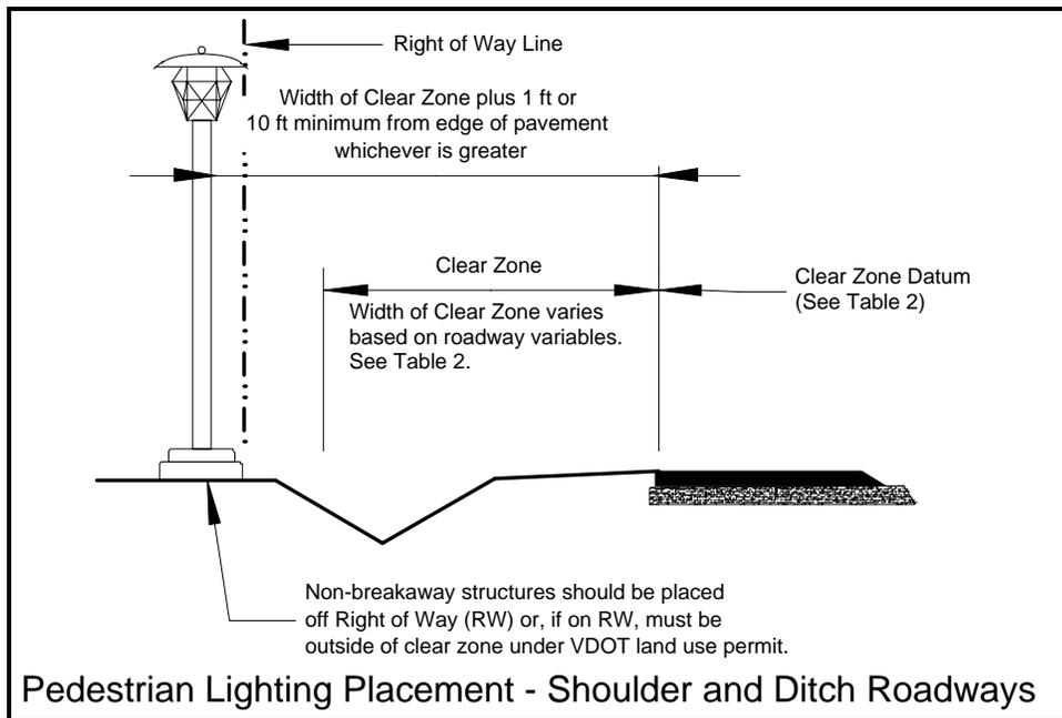
**FIGURE 15 – LIGHTING ALONG SHOULDER AND DITCH SECTIONS**
