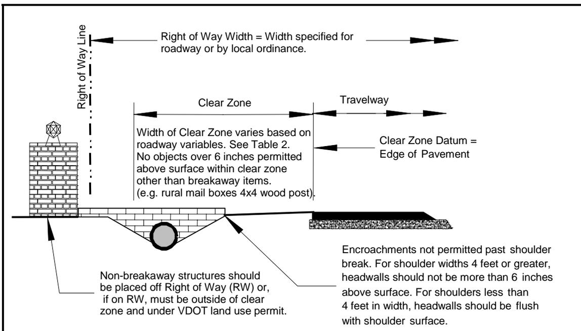
**FIGURE 11 – SETBACK DETAILS WITH SHOULDER AND DITCH**
