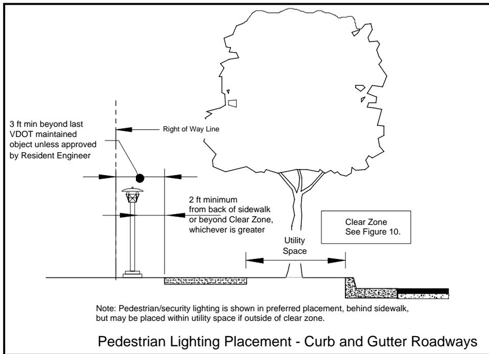
**FIGURE 14 – LIGHTING ALONG CURB AND GUTTER SECTIONS**
