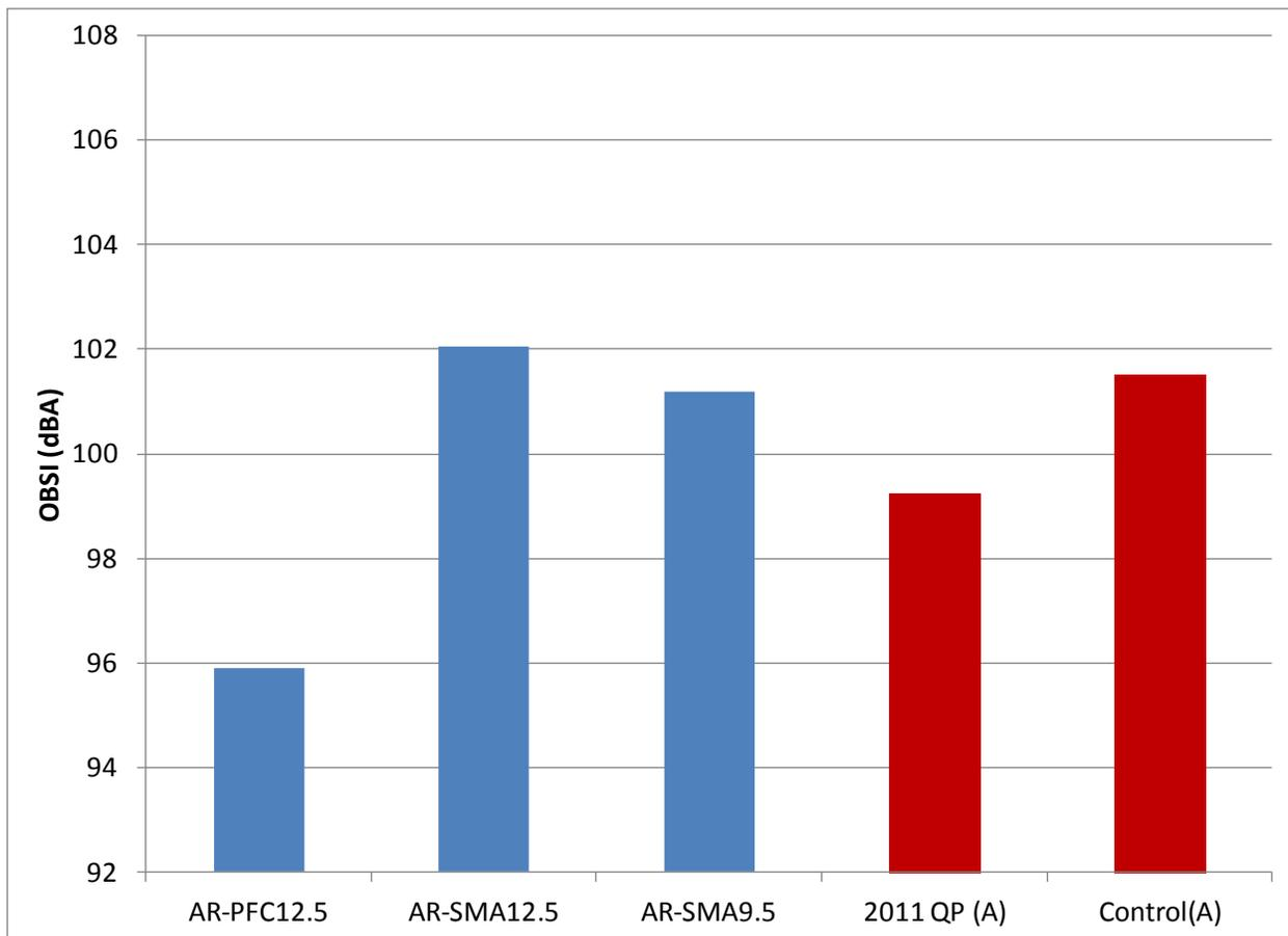
**Figure 4. Average OBSI Noise Measurements: 2012 Demonstration Materials (blue) Versus 2011 QP Materials and Overall Program Asphalt Control (red). OBSI = On-Board Sound Intensity; QP = quiet pavement.**
