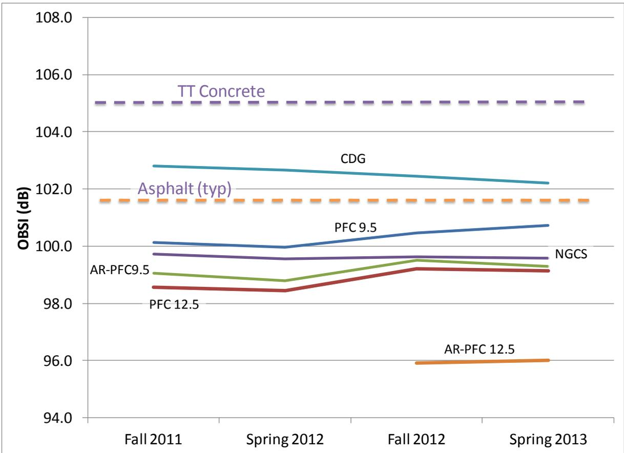
**Figure 5. OBSI Noise Value Trends With Time: Quiet Pavement Technologies and Typical Concrete and Asphalt Surfaces.** OBSI = On-Board Sound Intensity; TT = transverse tined; CDG = conventional diamond grind; (typ) = typical; PFC = porous friction course; NGCS = Next Generation Concrete Surface; AR = rubberized-modified asphalt.
